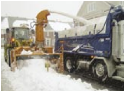
LARUE 3640 detachable snowblower, hydrostatic, 315 hp, 8500 lbs, 36 in. ribbon type screw, 40 in. turbine, telescopic chute
