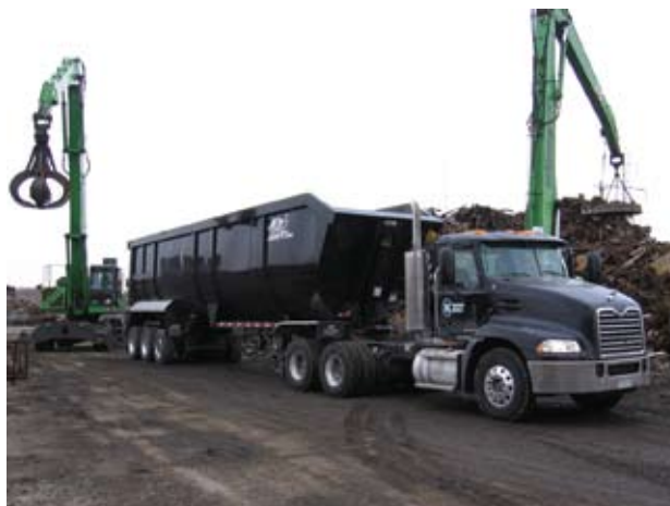
One of Niagara's Sennebogen 835 M machines is fitted with a 170 cm magnet, while the other has a grapple.
