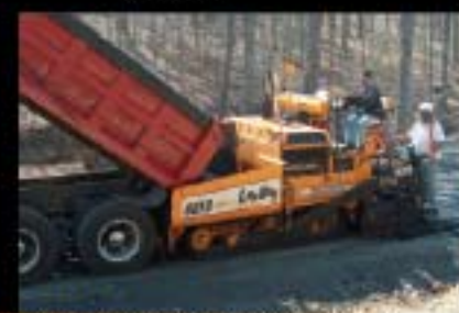
LeeBoy 8516 25,000 lbs class 8' to 16' paver Cummins 130 HP engine, Legend™ screed system with 10% slope or extensions, variable speed 14" cast segmented augers, patented under auger cut-offs.
