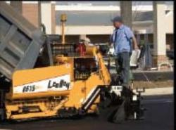
selboy 8816 25,000 lbs class 8' to 16' paver Cummins 130 HP engine, Legend\*\* screed system with 10% slope on extensions, variable speed 14" cast segmented augers, patented under auger cut-offs.
