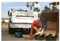
Powered by a 27 hp Kubota engine, EnPak eliminates the need for a PTO and integrates seamlessly into its electrical and fuel systems, allowing mechanics to run their tools with the truck's engine turned off.
