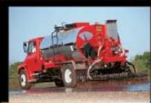
Rosco Meximizer III automatic In-cab controls, EZ Spray extendible spraybar, tapered and radius spraying, ENVI-RO-FLUSH clean-out system, straight-line start and stop, 8-20 ft spraybar available, 400 GPM Viking asphat pump
