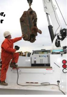
and accurate crane operation. And 6000 W of generator power at 100% duty cycle plus an additional 2400 W of pure sine wave EnVerter™ power at idle is available to run electrical tools including welders, lights and laptops used for equipment diagnostics.
