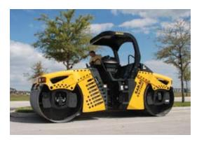
Sakai says the SW770 offers one frequency, 3000 vpm and two amplitude settings, low to high 0,03 to 0,063 cm, while the SW770HF offers a three frequency settings up to 4000 vpm, and the same amplitude settings as the SW770.
