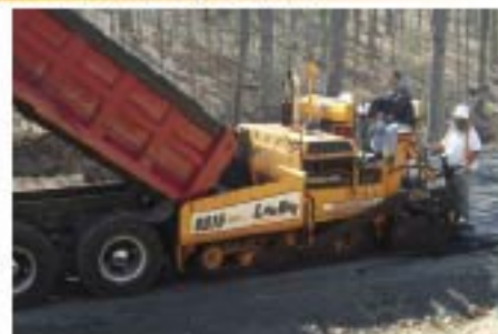
LeeBoy 8816 25,000 lbs class 8' to 16' paver Cummins 130 HP engine, Legend™ screed system with 10% slope on extensions, variable speed 14" cast segmented augers, patented under auger cut-offs.
