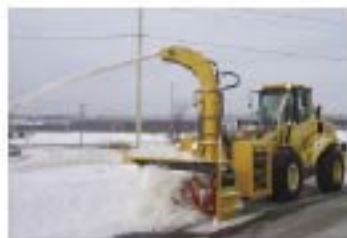
LARUE D55 detachable loader mount, mechanical drive, 300 HP, 8500 lbs, 36 in. ribbon auger, 40 in. impeller, telescopic chute.
