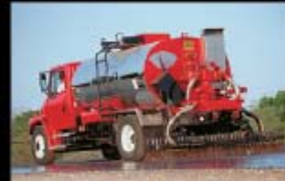
Rosco Roadbuilder II automatic in-cab controls, EZ Spray extendible sprayer, tapered and radius spraying, BW RW-FLUSH clean-out system, straight-line start and stop, 8-20 ft sprayer available, 400 GPM VMD asphalt pump
