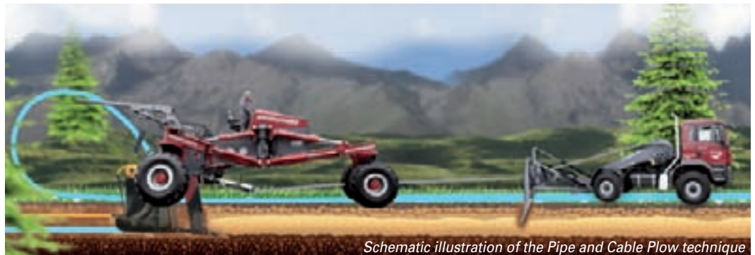
Schematic illustration of the Pipe and Cable Plow technique
