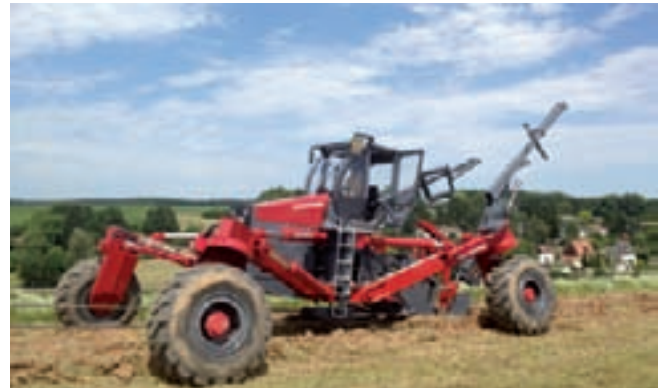
The SPIDER F 210 CAB for installing pipes and cables up to Ø 355 mm
