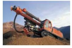
In Intermat 2003 **Sandik Tamrock** is presenting Axera T11 DATA, a computer controlled three boom electrohydraulic jumbo. It is designed especially for tunnelling and cavern excavation in 20-160 m<sup>2</sup> sections.
