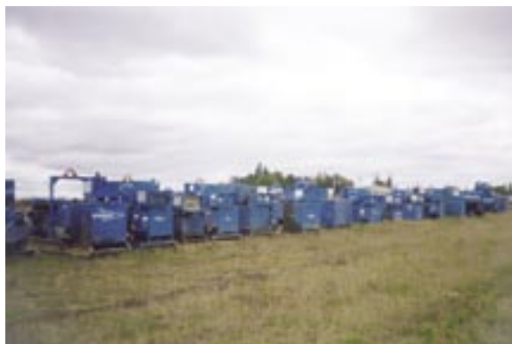
For the trench dewatering, the contractors used Flygt's BIBO pumps in sizes ranging from 2" to 8".
