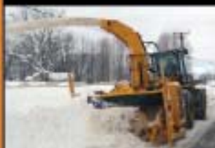
High capacity LARUE detachable loader-mounted, 200 hp or 350 hp, telescopic loading chute.
