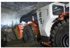
Like all Sandvik loaders, the 14 t electric-powered LHD incorporates key features of the recently launched diesel machines, such as upgraded cabin design and Vehicle Control and Management system (VCM). The electronic control system incorporates a state-of-the-art user interface with enhanced diagnostics and a platform for Sandvik's Automine technology, plus an upgraded electric system that are designed to interface optimally with the electronic control system.
