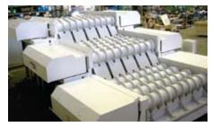
Such a system is of particular interest when weather conditions fluctuate, there can be changes in the H<sub>2</sub>0 content, and consequently in the screening behavior of the material to be processed. The gap setting adjustment facility provides the optimum means to compensate for any such variations during the screening operation.
