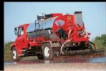
Rosco Maximizer III automatic in-cab controls, EZ Spray extendible spraybar, tapered and radius spraying, ENVI-RO-FLUSH clean-out system, straight-line staft and stop, 8-20 ft spraybar available, 400 GPM Viking asphalt pump
