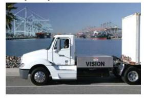
trucking environment. The Vision trucks are powered by a combination of a hydrogen fuel cell and lithium batteries and have a potential range of up to 645 km.
