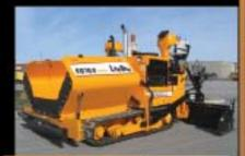
LeeBoy 8816B 25,000 lbs class 8 to 16 paver Cummins 130 HP engine, Legend™ screed system with 10% slope on extensions, variable speed 14" cast segmented augers, patented under auger cut-offs.
