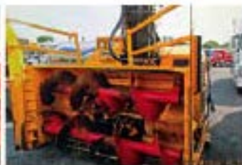
1999 VOHL DV-4000 , JD 275 hp engine, telescopic chute, ice screw, good condition .....
