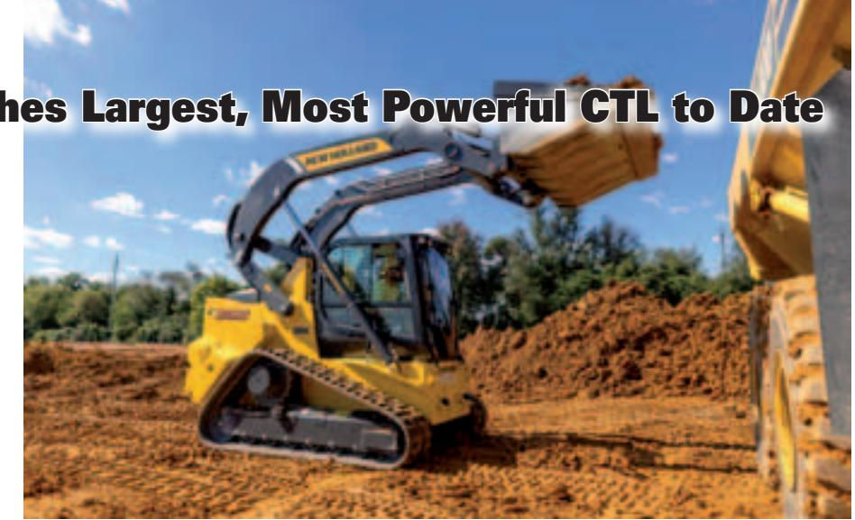
vertical lift design optimizes the C362 for lift-and-carry operations. With greater dump reach and height, customers can easily load high-sided truck boxes or hoppers. Full 360° visibility comes with the C362's low-profile Super Boom arm and shoulder design, an integrated rear camera, and new LED front work lights.
