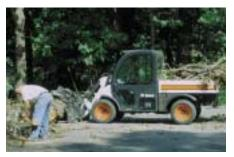
With four wheel drive and four wheel steer, the ToolCat is extermely versatile in a number of applications. It is probably the first of a new kind of compact equipment.
