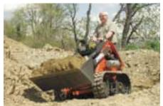
The **Ditch Witch SK500** is another of this new breed of multi-purpose machines. At only 36 inches in width, it can easily go through standard door openings. It comes with rubber tracks in order to minimize damages to pavement or grass.
