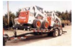
Landoll Corporation is one of the many manufacturers that offer those trailers. Used by contractors as well as equipment rental outlets, they feature tilting decks or sliding axles to facilitate the loading of low riding height equipment.
