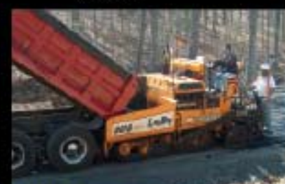
LeeBoy 8816 25,000 lbs class 8' to 16' paver Cummins 120 HP engine, Legend™ screed system with 10% slope on extensions, variable speed 14" cast segmented augers, patented under auger cut-offs.
