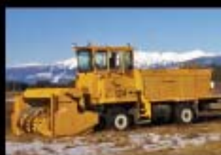
LARUE T460 dual engines, 775 HP, 4,400 tons/hour capacity, all wheel drive, available with the Larue A.R.S. (automatic rear steering all wheel steering system).
