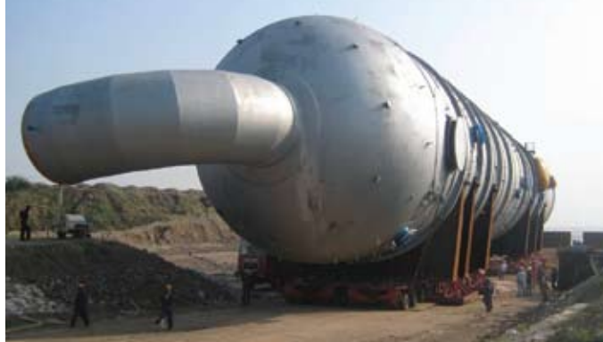
An additional 1,000 t rectification column on 48 NICOLAS MHD SPE axle lines.
