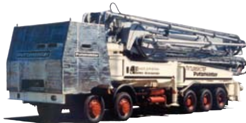
A truck-mounted concrete pump fitted with a lead cover for radiation protection as used in Chernobyl in 1986
