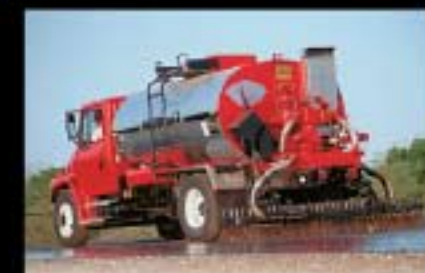
Rosco Maximizer II automatic in-cab controls, EZ Spray extendible spraybar, tapered and radius spraying, ENVIRO-FLUSH clean-out system, straight-line start and stop, 8-20 ft spraybar available, 400 GPM Viking asphalt pump
