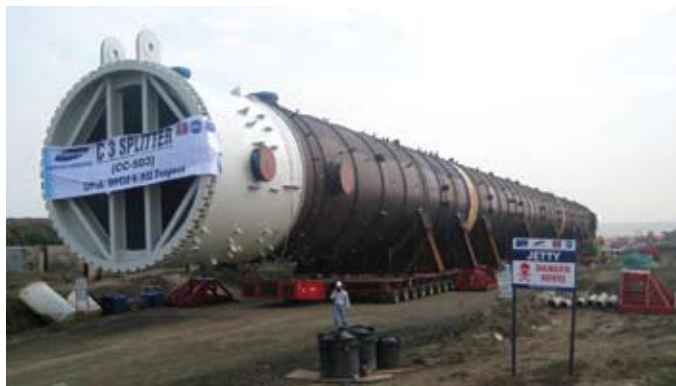
Roll-off of a 1,350 t rectification column with 64 NICOLAS MHD SPE axle lines. Transportation then continues along the final 1 km to the ethylene plant in Dahej.
