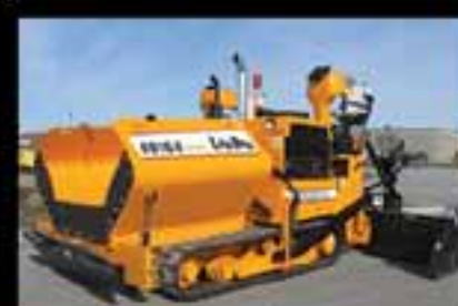
LeeBoy 8816B 25,000 lbs class 8' to 16' paver Cummins 130 HP engine, Legend™ screenshot system with 10% slope on extensions, variable speed 14" cast segmented augers, patented under auger cut-offs.
