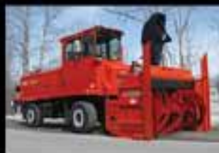
LARUE T85 dual engines: carrier 300 to 475 HP, blower head 665 to 1200 HP, 5,000 to 10,000 tons/hour capacity, all wheel drive, available with the Larue A.R.S. (automatic rear steering).
