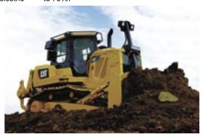
Optional AccuGrade™ grade control system can cut job costs significantly. Every D7E will come Grade Control Ready, which allows installation of the AccuGrade Attachment Ready Option at the factory or at the dealer.
