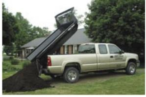
The insert comes in both 1,62 x 2,58 m (DI-100) and 1,62 x 1,93 m (DI-100-6) sizes and offers a rated lift capacity of 2700 kg. Due to its smaller, more compact size, the DI-100-6 holds a volume of 1,14 m $^3$  while the DI-100 transports up to 1,52 m $^3$ . A Bri-Mar dump insert becomes an invaluable tool for any landscaper, renovation contractor, roofing & siding contractor or homeowner with a pick-up truck.
