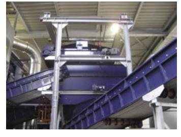
At a later state, all non-ferro metals such as aluminium, copper and brass are removed from this building and demolition waste. At IFAT the firm from Waalre presented, among other things, magnetic systems and non-ferro separators.
