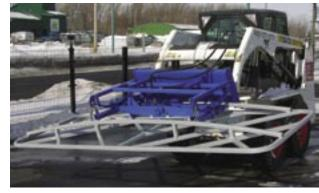
This product redefines conventional methods for leveling work. The latest version of the leveling grid allows swiveling using a hydraulic cylinder, without affecting the flexibility for which this product is reknowned.
