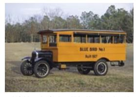
wood deteriorated before the customer could finish paying for the vehicle. Albert Luce investigated ways of building a better bus and constructed a body using steel angles and channels, steel sheets, wood and canvas. He then mounted it to a 1927 Ford Model T chassis. This new bus was sold to Frank Slade of Marshallville, Georgia to be used as a school bus.
