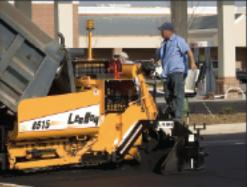
LeeBoy \$816 25,000 bs class 8' to 16' paver Cummins 130HP engine, Legent "\* screet system with 10% slope
