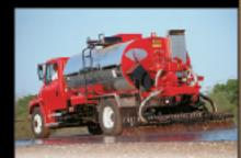
Rosco Hadmitrer III automatic in-cab controls, EZ Spray extendible spraybar, tay ered and radius spraying, BW RO-FLUSH clean-out system, straight-line start and stop, 8-20 ft spraybar available, 400 GPM Widing asphalt pump
