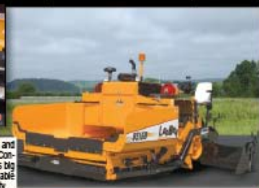
LARUE T60 self-propelled, hydrostatic drive, Cat 375 HP engine, ribbon or dual auger configuration, available with the Larue A.R.S. (automatic rear steering) and telescopic chute.
