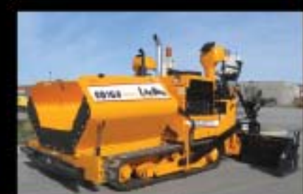
LeeBoy 8816B 25,000 lbs class 8' to 16' paver Cummins 130 HP engine, Legend™ screenshot system with 10% slope on extensions, variable speed 14" cast segmented augers, patented under auger cut-offs.
