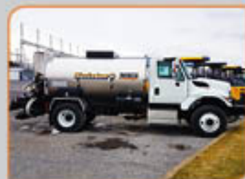
Asphalt distributor Rosco Maximizer 3 1900 gallons Mounted on truck International 7300
