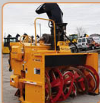
Snowblower Larue D65 2017 USED Ribbon of 40 inches engine 365 hp From 270 to 380 hours
