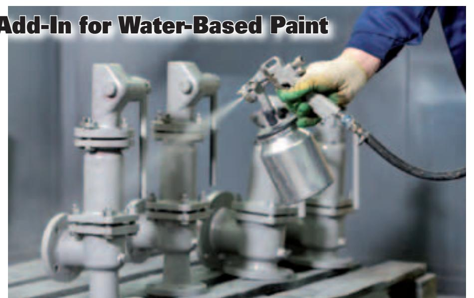
corrosion – which is a common problem for water-based coatings – and has the ability to reduce scribe creep – a standard test method used to measure corrosion when coated panels undergo salt spray or humidity testing.
