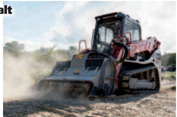
tors that delivers excellent productivity, with low noise and vibrations. It effortlessly crushes rocks and hard surfaces such as bitumen, asphalt and concrete. Most common applications for this attachment include trenching in hard compacted material, profiling of rocky or concrete walls for foundations and tunnels, mountainside excavation for hilly road construction, quarrying and underwater dredging.
