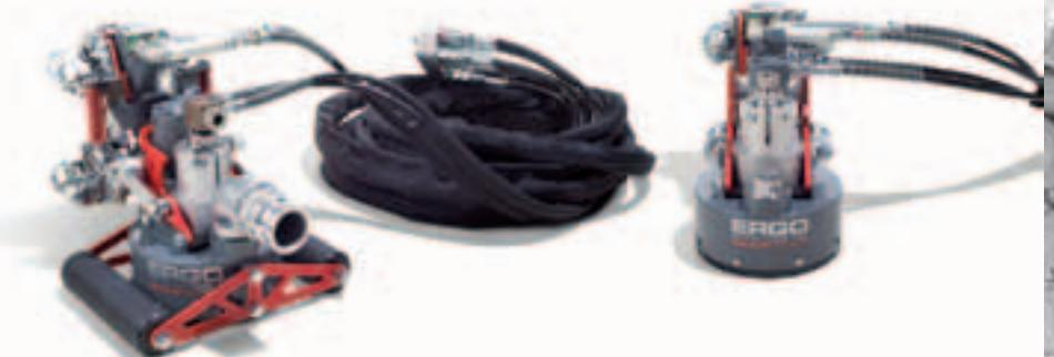
The Ergo System also works with Rotolance attachments for improved capabilities in confined or hard-to-reach places. The Ergo Rotolance 130 and 130S work at pressures ranging from 1,000 to 3,000 bar and offer a variety of nozzle configurations for a spray pattern diameter from 30 mm to 130 mm.
