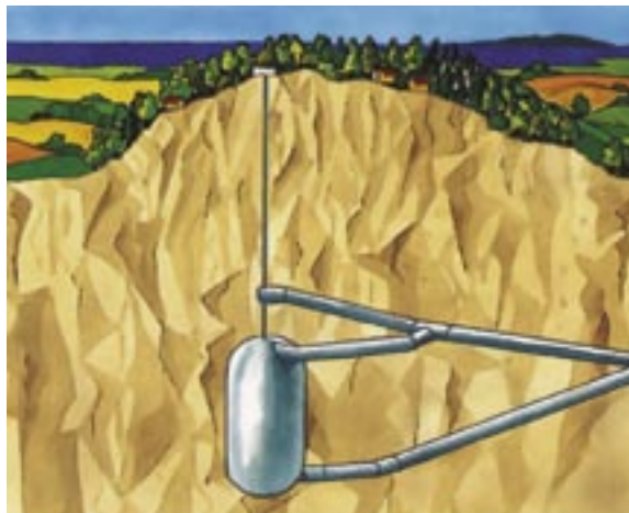
The steel cylinder can withstand pressure of 200 bar, or 200 times atmospheric pressure.
