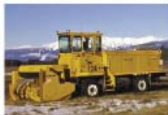
LARUE 7460 dual engines, 775 HP, 4,400 tons/hour capacity, all wheel drive, available with the Larue A.R.S. (automatic rear steering all wheel steering system).
