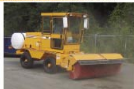
Resco Challenger III Heavy-Duty broom for the most demanding jobs. Quick change brush core (less than 5 minutes to change), 80 hp Cat power, hydrostatic drive, R.O.P.S. pressurized air conditioned cab.
