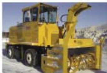
LARUE T60 self-propelled, hydrostatic drive, Cat 375 hp engine, ribbon or dual auger configuration, available all wheel steer and telescopic chute.
