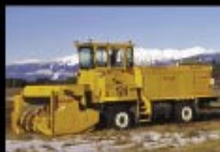
LARUE 7450 dual engines, 775 HP, 4,400 tons/hour capacity, all wheel drive, available with the Larue A.R.S. (automatic rear steering all wheel steering system).
