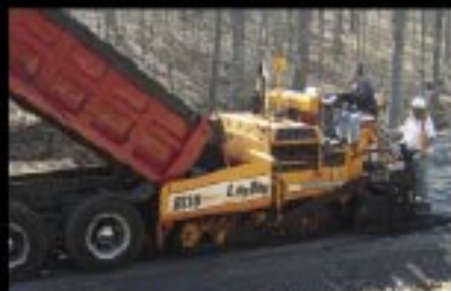
LeeBoy 8515 25,000 lbs class 8' to 16' paver Cummins 130 HP engine, Legend™ screed system with 10% slope or extensions, variable speed 14" cast segmented augers, patented under auger cut-off.
