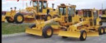
LeeBoy 785 Grader All-gear Drive built-in drive, 130 HP Cummins engine, 25,300 lbs static weight, 6 speed forward / 3 speed reverse powershift transmission, 12 foot self-lifting moldboard, articulated frame 40°.
