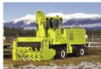
LARUE 7060 single engine 550 HP, hydrostatic drive, 4,000 tons/hour capacity, available with the Larue A.R.S. (automatic rear steering all wheel steering system).
