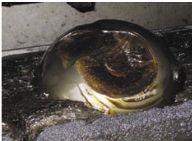
Chipped slew ball from the the giant machine's slewing ball race.
