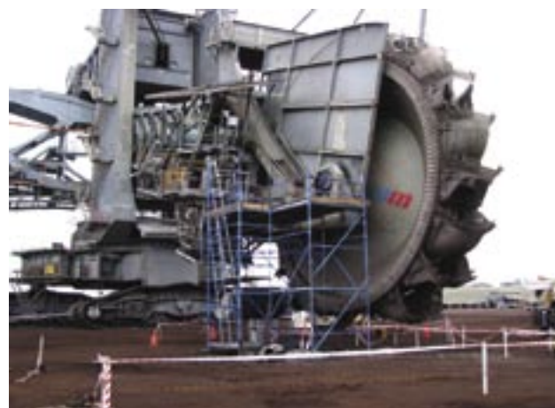
Dredger 16 weighs a total of more than 5000 t and can remove 60 000 t of overburden a day.
