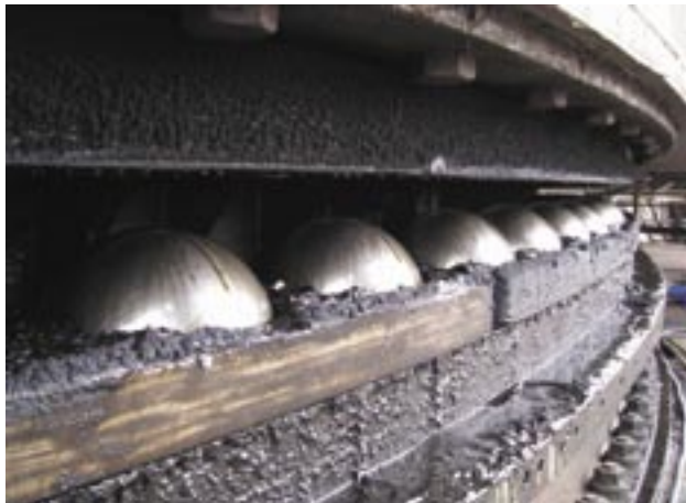
The dredger has a slew ring bearing 15,2m in diameter containing 177 balls of 200 mm diameter each weighing 32 kg.
