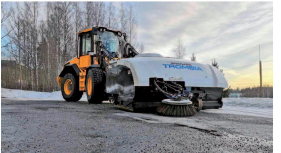
Trombia sweeper attachments are completely filter-free and use a globally patented technology that combines airknife dust removal, mechanical sweeping, vacuum and cyclone separation. Inside Trombia's sweeping chamber the sweep-
