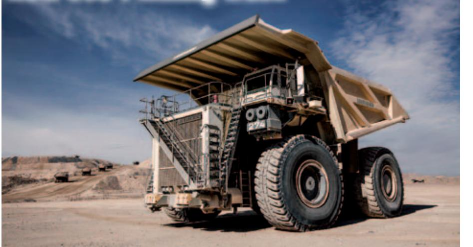
Liebherr recently launched the T 274, a 305 t haul truck. It bridges the gap between the highly successful T 284 (363 t) and the upgraded T 264 (240 t).
