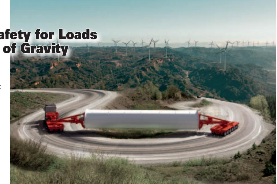
(loaded) or 910 mm (unloaded) which makes driving under loads easier. The high axle compensation of 680 mm also makes driving on uneven surfaces safer. Moreover, the maximum steering angle of +/- 60° ensures optimal maneuverability. Lifting and lowering is carried out with the help of a low-emission Power Pack Unit (PPU) from the Z19 series.
