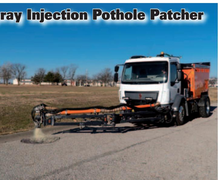
volumetric capacity is 3.8 m<sup>3</sup>. A 55° hopper wall angle allows material to flow steadily to the augers, eliminating the need for a vibration system. And in a feature exclusive to the SP5E, aggregate can easily be unloaded from the hopper by removing a cover in the rear and operating the auger(s) in reverse.
