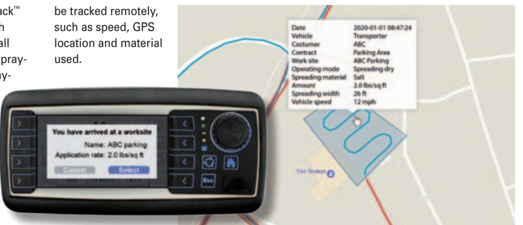
Geofencing capabilities allow users to remotely create work sites for different client areas, as well as set application rates for each client's site according to weather conditions. With this information entered into the system, the StrikeSmart controller alerts drivers which sites to treat during winter events, and it recognizes when the driver enters each work site. Then, the spreaders and sprayers automatically
