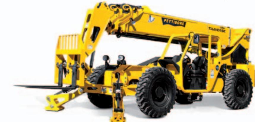
ward reach to 14 m. Delivering a maximum load capacity of 4,500 kg, the telehandler is powered by a 117-hp Cummins QSF 3.8 diesel engine. Mounted on a side pod, the engine offers easy service access while allowing excellent curbside visibility and ground clearance of 45 cm.
