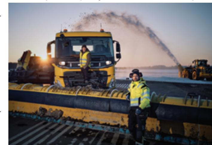
Given the easy-to-service nature of the D11 range and its proven compact base engine development, instances of prolonged or unexpected downtime are rare. Additionally, Øveraasen makes doubly sure its machines provide instant availability by choosing engine packages equipped with a pre-heater that support engine starting in ambient temperatures below -15°C.
