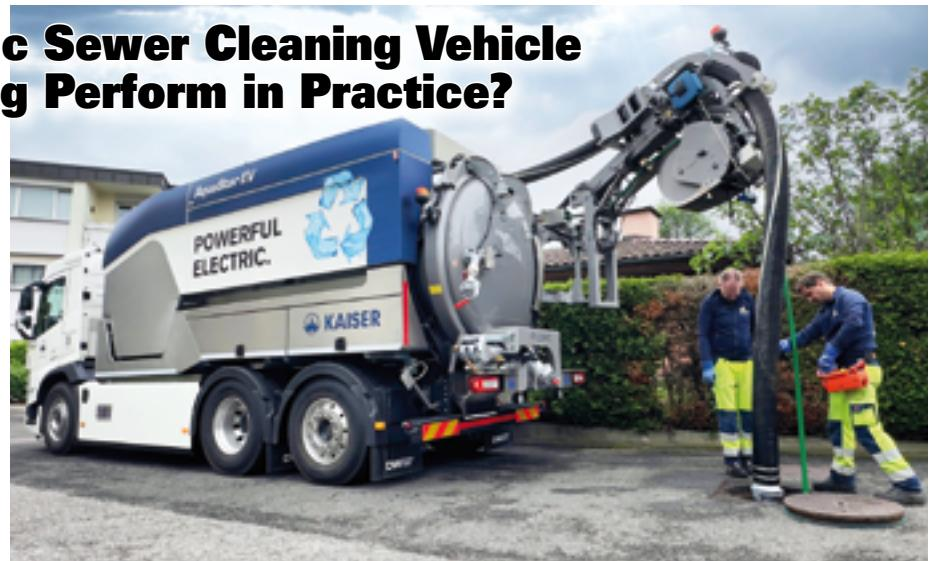
An electric sewer cleaner would be particularly well suited for jobs in urban areas, where recharging is easier to plan. The electric truck is then on a level playing field with the diesel vehicle and even has some advantages over it. Particularly with combined jetting and recycling, you notice that the electric truck is a lot quieter which makes the work more pleasant for the operator and for the residents.
