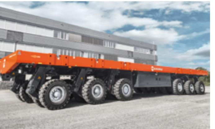
lines and accommodating payloads of up to 256 t, are used at Geneva Airport. The runway there is constantly being refurbished. Concrete slabs, each measuring 15 x 8 m and weighing 180 t, used to create the runway, are being replaced one by one with new prefabricated slabs.
