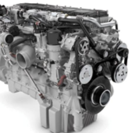
at an injection pressure of 2,500 bar. This makes it one of the systems with the highest pressures on the market and guarantees optimum fuel atomization quality. As a result, significant savings in fuel consumption can be achieved.
