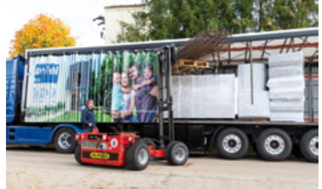
With its maximum lifting capacity of 2,100 kg, the BM 214 truck-mounted forklift can also handle heavy loads. It owes its excellent off-road capability to permanent all-wheel drive combined with compact dimensions. Because it is housed inside the transport box, the BM 214 remains protected from salt water and dirt in winter.
