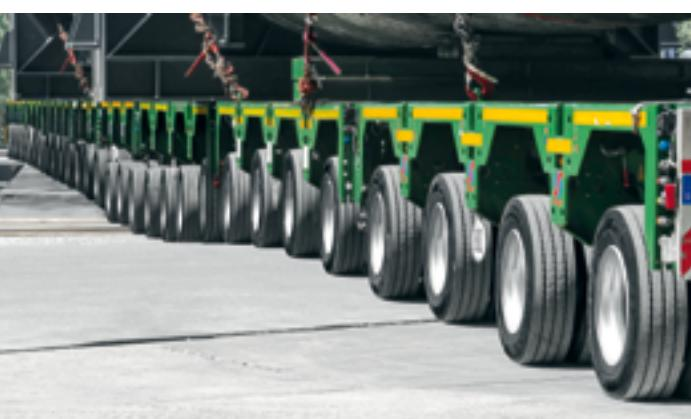
the case of the U17 transport, InterCombi vehicle combinations can not only be used as trailer combinations but also as tractor-trailer combinations or as self-propelled transporters.
