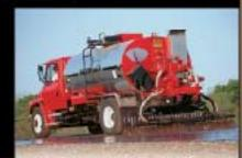
Rosco Madunter III automatic in-cati controls, EZ. Spray extendible sprayter, tapered and radius spraying, EW RO-RLUSH clean-out system, straight-line start and stop, 8-20 ft sprayter available, 400 GPM Widnig asphalt pump.
