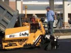
LeeBoy 8816 25,000 bis class 8" to 16" paver Curmins 130 HP engine, Legend" screed system with 10% slope on entersions, variable speed 14" cast segmented augers, patented under auger cut-ofts.
