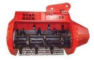
The Compact Equipment Mulcher offers a 91 cm cutting width and a maximum weight between 450-550 kg. Targeted for excavators in the 7-12 t range with 17-30 gpm of auxiliary flow. The Compact Equipment Mulcher also works well on other applicable machinery such as larger back hoes.
