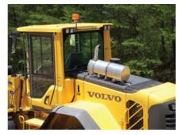
CARB Level 3+ requirements. Volvo equipment owners can utilize the system to help comply with the "In-Use Off-Road Diesel Vehicle Regulation", or to provide the best available control technology (BACT) for the newest machines in owners' fleets. Previously, engines using any type of EGR had been excluded from applying exhaust retrofit technology in California. This has now changed with the recent system verification by the state.
