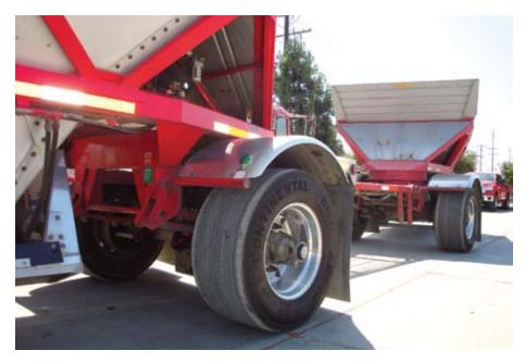
agreed the HTL1®'s advantages of both weight savings and stone ejection make this tire ideal for the trailer position in construction and on/off road applications.
