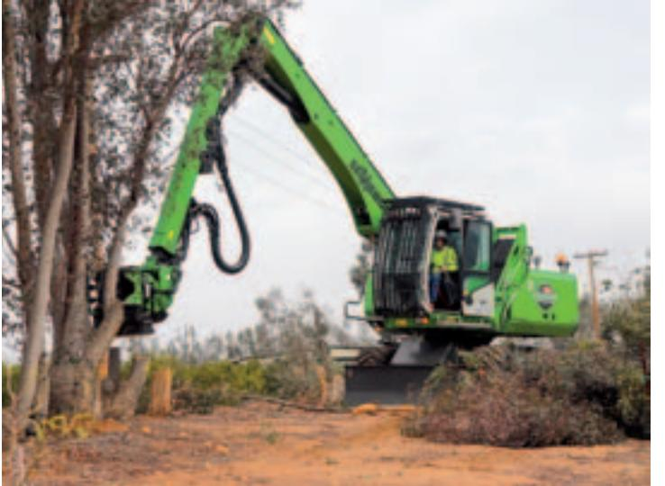
saw attachment. Its powerful hydraulics are tuned for delicate tree trimming as well as heavy cutting. With its 1,700 kg lifting capacity, the 718 easily grasps, cuts, moves and stacks whole trees and large limbs in a single smooth movement.
