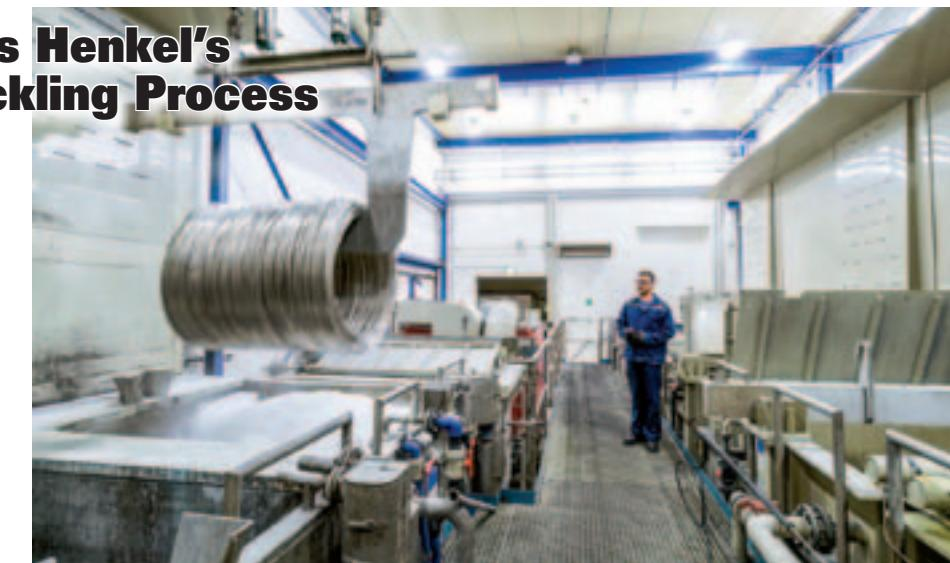
chemical and appliances sectors. But there are challenges around common mixed acid pickling systems, due to the use of nitric acid. These cleaning techniques typically result in vast volumes of nitrate ions being discharged, during the intermediate and final rinsing stages. Nitrate and nitrite pollution is subject to legislative regulation and needs to be complied with via waste water treatment.
