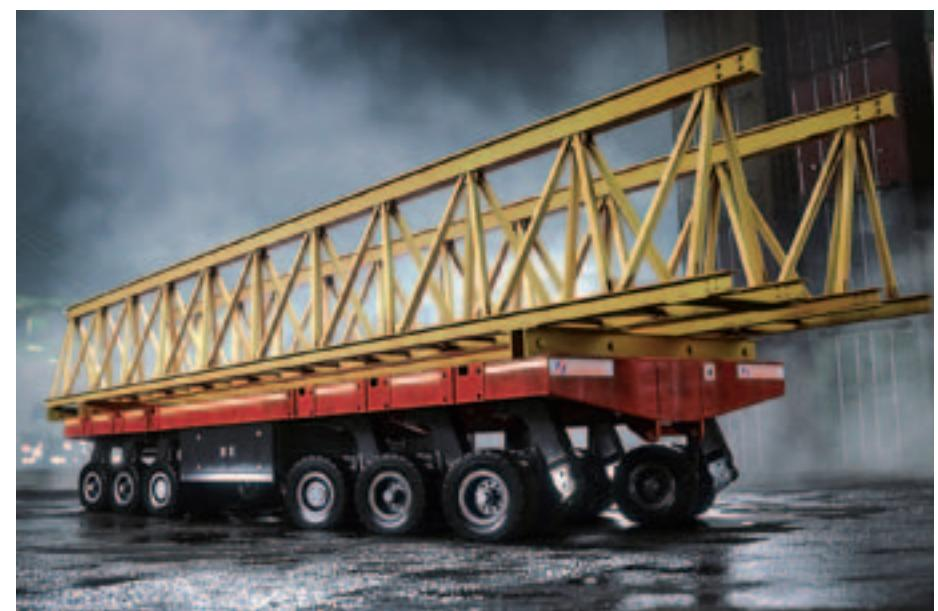
and safe to operate but it can also be used on a wide range of surfaces both outdoors and in production halls regardless whether the road surface is made of gravel, asphalt, concrete or similar materials. For this reason and due to the high degree of axle compensation in the pendulum axle bogie unit, reloading is not required when transporting from a building into open spaces. This makes the self-propelled
