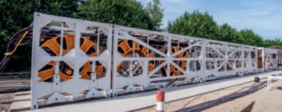
existing microtunnel or auxiliary tunnel. The actual work is carried out underground, essentially invisibly. The electric drive system also considerably reduces the ecological disturbance of a cutting site. When it comes to logistics, the system's compact dimensions are a major advantage. The BAUER Cube System is as easily transported to its place of deployment as
