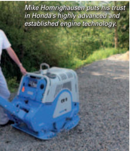
working width can be extended to 90 cm, and it has an operating speed of up to 28 m/min. The CR 9 Hd CCD version also includes the COMPATROL compaction control system.
