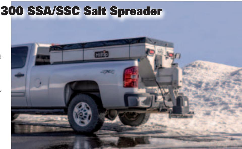
All models include a stainless steel flip-up chute designed to spread salt in environments with high humidity, and a tarp kit to help keep spreading materials dry.
