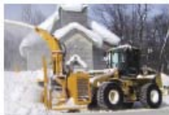
High capacity LARUE D55 & D65 detachable loader-mounted, 300 or 350 hp, telescopic loading chute.
