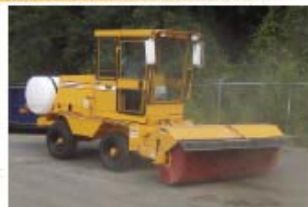
Rosco Challenger III Heavy-Duty broom for the most demanding jobs. Quick change brush core (less than 5 minutes to change), 80 hp Cat power, hydrostatic drive, R.O.P.S. pressurized air conditioned cab.
