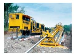
Vermeer Corporation has expanded its complete line of NAVIGATOR® horizontal directional drills with the introduction of three maxi-sized drill rigs – D500x500, D750x900 and D1000x900 – designed specifically for large diameter pipe installations. The new units feature pullback forces of 225 000 kg, 337 500 kg and 450 000 kg.
