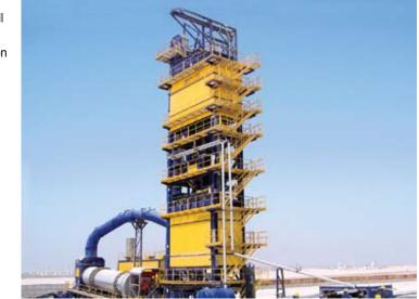
The plant will be producing up to 240 tonnes of asphalt per hour for the construction of the track surface.
