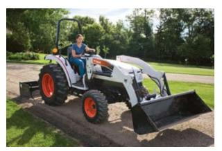
The Bobcat compact tractors feature fourwheel drive for traveling over and working in rough terrain, and also come with hydrostatic transmissions for easy operation.
