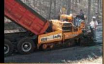
LeeBoy \$\$16,25,000 b: class \$' to 16' paver Curamins 120HP engine, Legend"\* screed system with 10% slope on extensions, variable speed 14" cast segmented augers, patientist under auger cut-offs.
