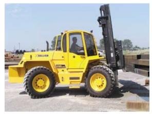
fully automatic power-shift transmission for efficient operation. Axles feature enclosed wet disc brakes for extended life, and limited slip differentials for maximum traction and maneuverability.
