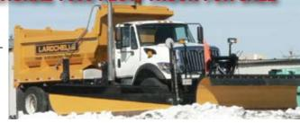
All new LAROCHELLE snow & ice removal equipment: 14' U-shaped dump-spreader (front discharge spreading), trip edge reversible plow with quick hitch, patrol wing with travel positionner, pre-wet system (1200 liters), electronic spreading control and in-cab air controls......Priced to sell Contact Larochelle Equipment Inc. at 418-522-8222 or visit www.larochelle.ca
