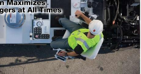
cause mix to push forward under the paver. If there is too much or too little material around the auger, problems in the paved surface will result. Paving speed, flow gate settings, and feed sensor position regulate material flow. Being able to easily see the augers allows the operator to monitor these variables and to deliver mix evenly across the augers and thus across the entire leading edge of the screed plate, which is a requirement for a segregation-free mat.
