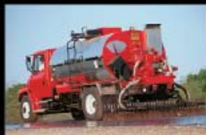
Rosco Modinizer 81 automatic in-cab controls, EZ Spray extendible spraybar, tapered and radius spraying, BW 40-FLUSH clean-out system, straight-line start and stop, 8-20 ft spraybar available, 400 GPM Viking asphalt pump
