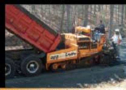
LeeBoy 8516 25,000 lb class 8' to 16' paver Cummins 130 HP engine, Legend™ screenshot system with 10% slope on extensions, variable speed 14" cast segmented augers, patented under auger cut-offs.
