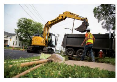
able with an optional offset boom which increases stability and maneuverability while working in confined areas, such as next to walls or close to traffic.
