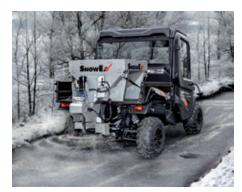
SnowEx® offers a new 0.27 m³ stainless steel spreader developed specifically to fit UTVs and compact trucks. The advanced corkscrew, or "helix" design of the HELIXX spreader helps prevent clogs and outperform the material flow of traditional augers.
