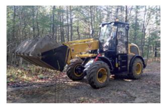
diesel engine developing 50 hp and 74 hp respectively, a 2-speed hydrostatic transmission and come with a comprehensive cold-weather kit. Conventional mechanical joysticks and a minimum of electronic increase the reliability of the unit. To insure a long life and high reliability, all liquids and lubricants used on all machines are made by Petro-Canada distributed by Petro Sherbrooke.
