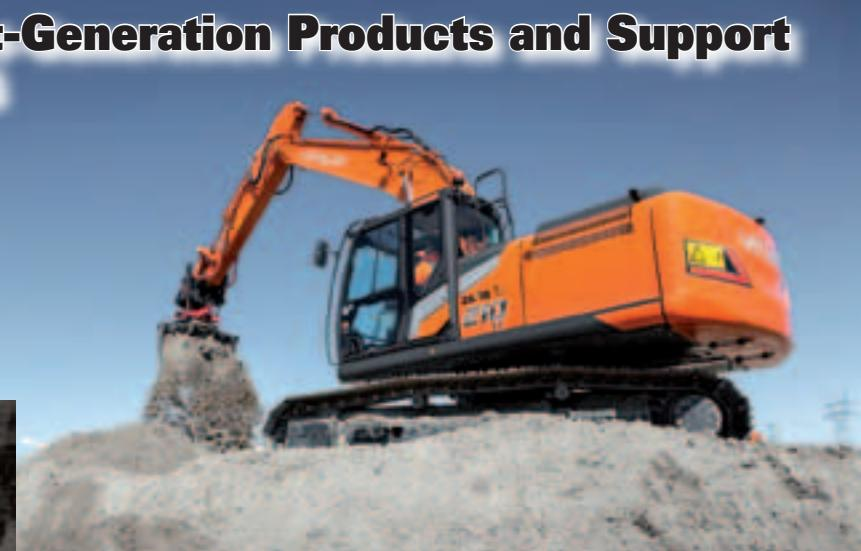
TRIAS III – features a unique 3-pump system to enhance productivity and efficiency on the ZX210-7, ZX245-7, ZX300-7, ZX345-7 and ZX350-7 excavators. The TRIAS III system allows the 3 hydraulic pumps to work together and direct oil flow for maximum efficiency of the bucket, arm and boom.
